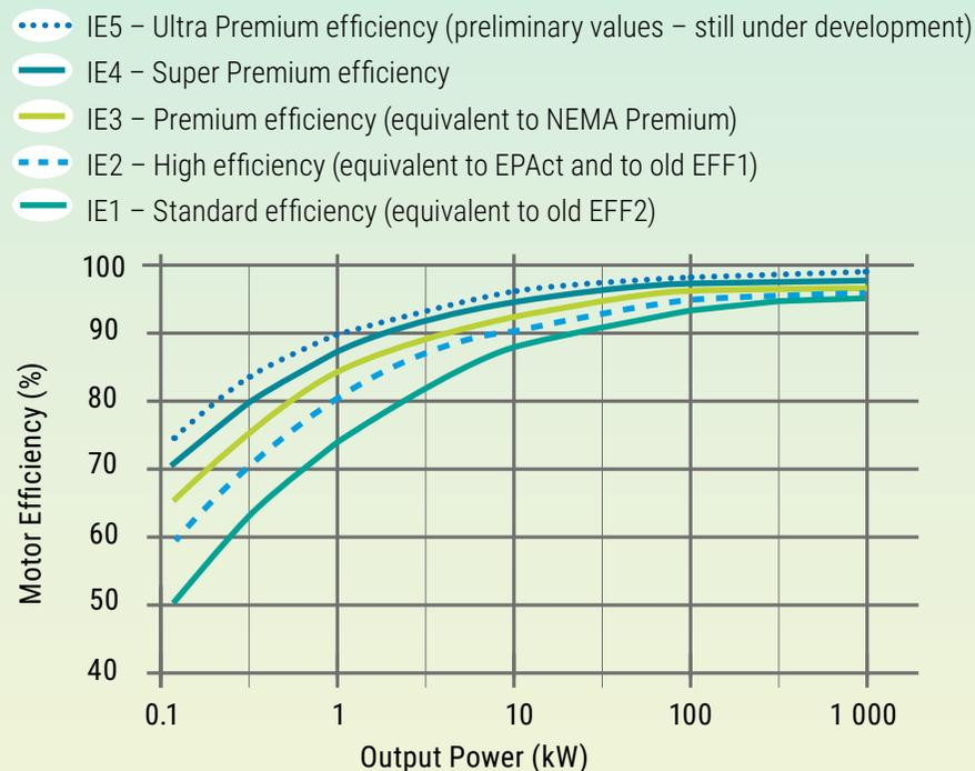
Figure 2: Induction Motor Efficiency Classification IEC 60034-30-1 {2014} – (UNIDO, 2012)
