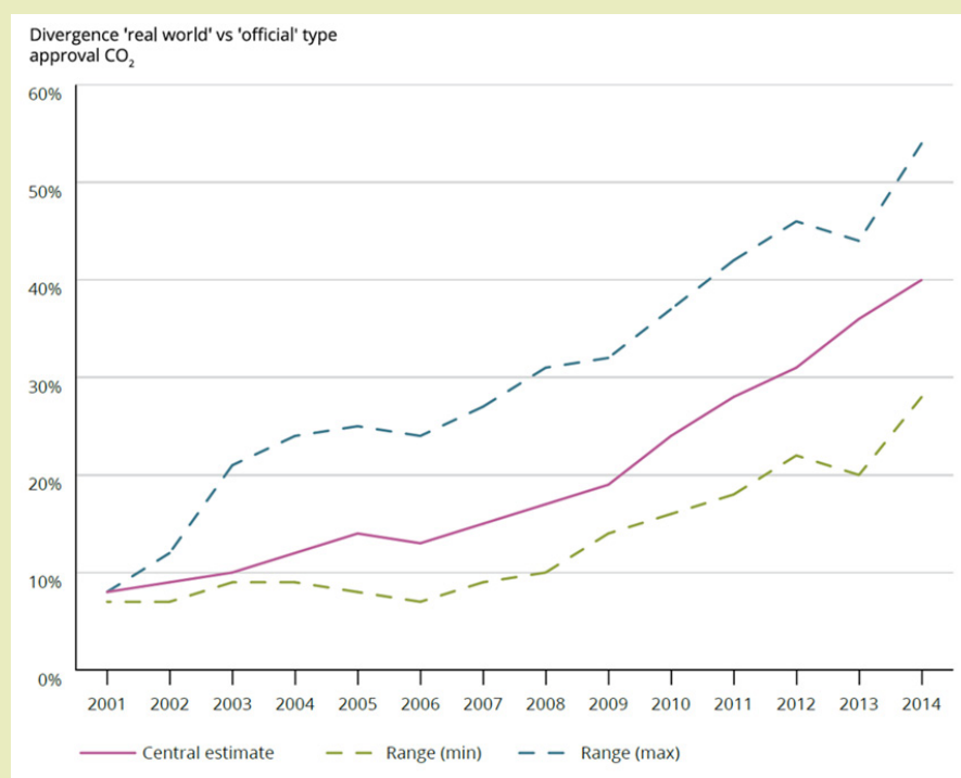
Figure 36: Divergence of real-world CO 2 emissions from manufacturers' type approval CO 2 emissions
