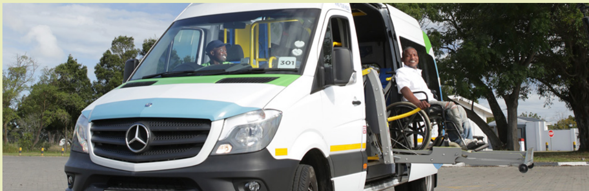
Figure 39: Converted Minibus Taxi developed by DBSA for Go George Integrated Public Transport Network
