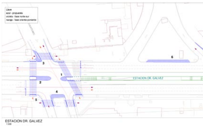
Fig. 13.36 A redesigned intersection in Mexico City for safe BRT access. The medians have been extended into the intersection to reduce turning speeds and provide more pedestrian refuge, and crosswalks brought into line with actual observed pedestrian movement.
