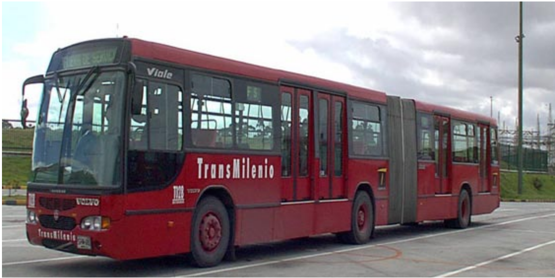
Fig. 12.18 Bogotá utilises a four door configuration that helps to reduce boarding and alighting times.
