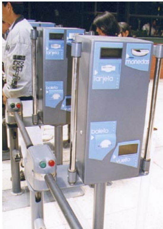
Fig. 12.54 This fare verification machine in Quito handles both coins and a magnetic strip fare card.
