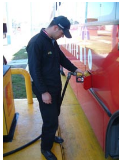
Fig. 11.106 and 11.107 Upon entering the re-fuelling area, a digital monitoring device (left photo) records the pertinent vehicle details (e.g., fuel level, odometre). If fuel is required, an attendant will then re-fuel the vehicle (right photo).
