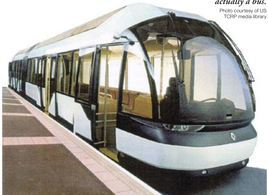
Fig. 12.39 Despite giving a distinctly light rail appearance, the Cibus vehicle is actually a bus.
