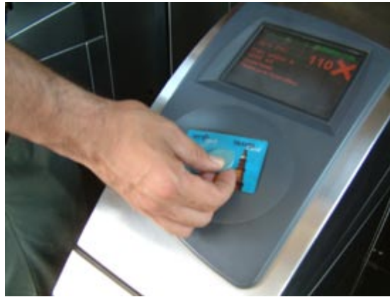
Fig. 12.52 and 12.53 The Delhi Metro utilises both smart card technology and electronic token technology. The smart cards allow multiple trips while the token is for single trips.
