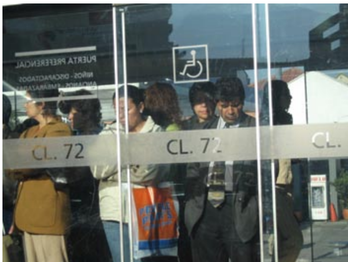
Fig. 11.61 and 11.62 Sliding station doors serve several functions including customer safety, climate control, and fare evasion.
