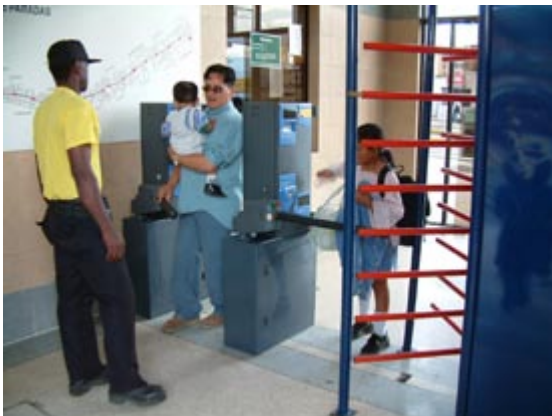
Fig. 12.66 The gate-arm turnstile as used in Quito can be quite user-friendly, but does tend to increase the risk of fare evasion.
