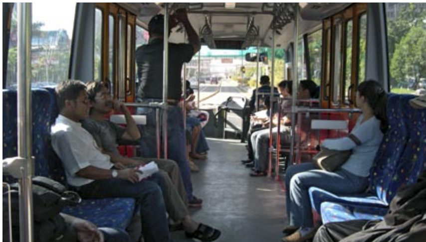
Fig. 12.17 Side facing seating, as shown in this example from Jakarta, will tend to maximise space for standing passengers and thus such a configuration will maximise overall passenger capacity per vehicle.
