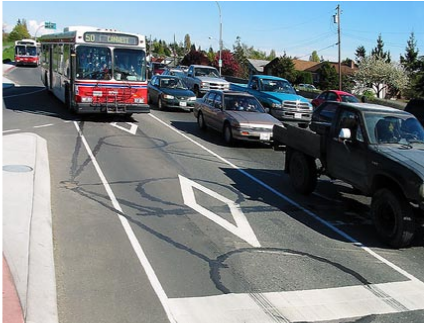
Fig. 11.128 In North America, queue-jumping lanes are used to give preferential treatment to buses at intersections.
