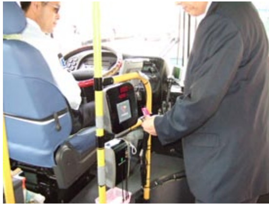
Fig. 8.17 and 8.18 The Seoul busway system uses smart card technology for fare collection (left photo). However, the on-board nature of the fare verification means that dwell times are negatively affected. A single passenger searching through personal effects for their smart card can create a significant delay (right photo).
