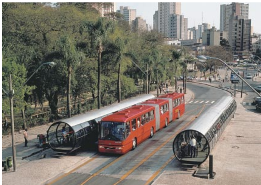
Fig. 8.15 Curitiba's innovations with station design and the station-to-vehicle interface did much to make BRT a high-capacity option. Photo courtesy of Volvo
