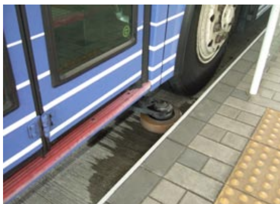
Fig. 5.33 and 5.34 Nagoya’s elevated BRT line utilises a mechanical guidance system to reduce the required roadway width.
