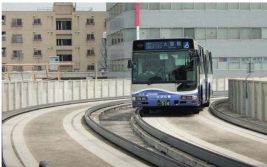
Fig. 5.33 and 5.34 Nagoya’s elevated BRT line utilises a mechanical guidance system to reduce the required roadway width.
