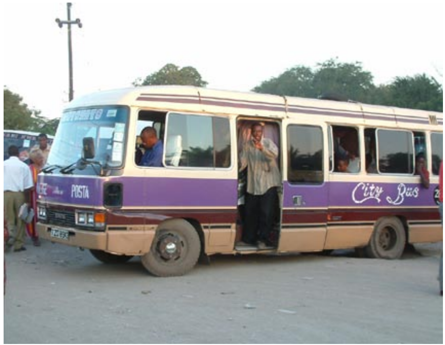
Fig. 4.21 Collecting data on origins and destinations and fares paid from passengers using the Dar es Salaam “Daladalas” helped to define the operational characteristics of the proposed BRT system.
