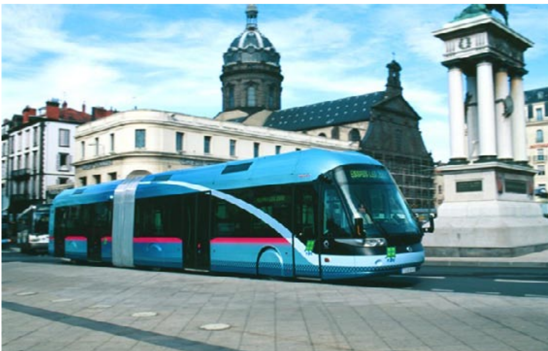
Fig. 2.55 Modern vehicles can give BRT systems a highly professional image. The vehicle in this photo is a Civis bus and not a light rail vehicle.
