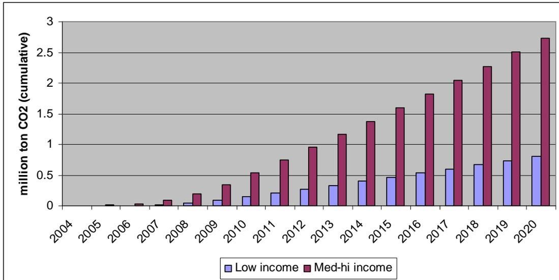
Figure 31: Cumulative CO<sub>2</sub>-eq emission savings for the residential lighting scenario relative to the reference case
