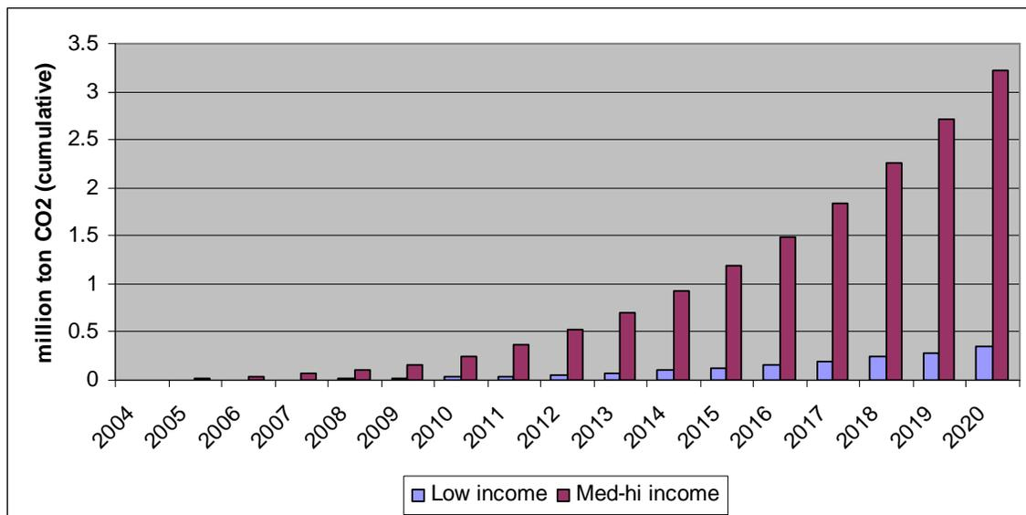
Figure 29: Cumulative CO<sub>2</sub>-eq emission savings from a solar water heater programme in the residential sector
